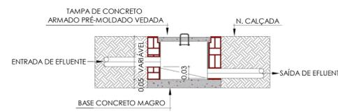
DETALHE CX. DE INSPEÇÃO E PLUVIAL (C.I./C.P.)
